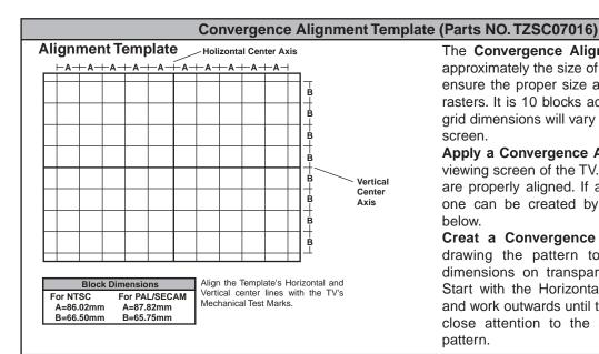
The **Convergence Alignment Template** is a grid approximately the size of the viewing screen used to ensure the proper size and shape of the alignment rasters. It is 10 blocks across by 8 blocks high. The grid dimensions will vary according to the size of the
